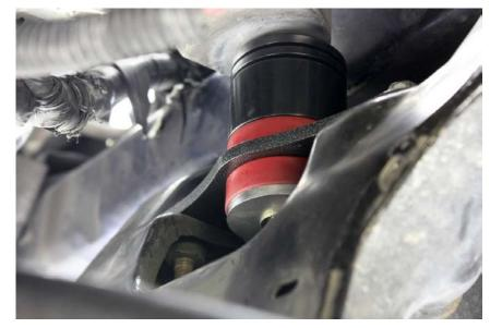
Assemble them as shown on the following page then bolt them to the K-member. Torque the mounting bolts to 41 ft/lbs.
