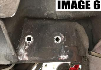
9. Reinstall reinforcement brace.
