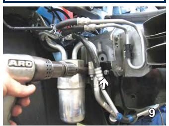
9. On the passenger side, align the baseplate with the existing hole, be sure the baseplate is level and clamp in place with the large vice grips. Using the baseplate as a template, drill the additional three holes with the 13/32" drill bit. In order to protect the hoses, put a tube over the drill.
