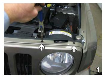
Remove seven bolts with a T20 Torx from across the top of the fascia (driver's side shown in photo). Set bolts aside to be reinstalled later.
