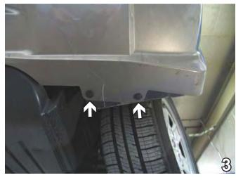
Under the fascia remove the two pushpins in front of the tire. Do this to both sides of vehicle. Set pushpins aside to be reinstalled later.
