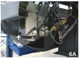
On the driver's side, remove the two Christmas tree pins and unplug the horn. Using a 13MM socket, remove the two bolts (gray arrows). Set bolts aside to be reinstalled later.
