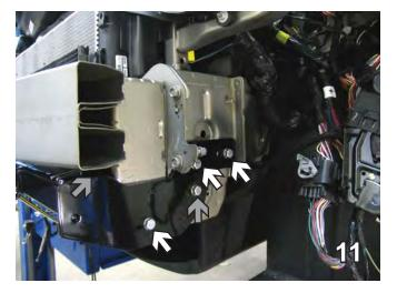
11. On the driver's side, install 3/8 x 1 1/2" bolts with 3/8" lock washers and tighten to 3/8-16 nut plates (white arrows). The top two nut plates are inserted from the front (see gray arrow on photo in step 8 for opening) and the bottom two are inserted from the bottom. Install the 1 x 1 1/2" spacer plate between the baseplate and the frame (gray arrow) and install 3/8 x 2" bolt with 3/8" lock washer and 3/8-16 nut plate. Use Loctite Red on all bolts.
