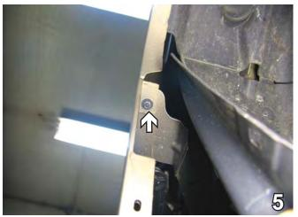
5. In front of the tire pull the wheel well cover back to remove the bolt with a 7MM socket. Do this on both sides. Set the bolt aside to be reinstalled later. Pull forward on the fascia to remove it, disconnect the turn signals and running lights (if applicable). Do this on both sides. Set the fascia aside carefully to be reinstalled later.
