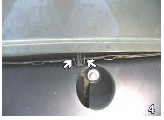
4. In the middle under the fascia, remove the two clips by pushing the sides of the clip together with a small screw driver. Set the clips aside to be reinstalled later.
