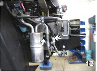
12. On the passenger side, install 3/8 x 1 1/2" bolts with 3/8" lock washers and tighten to 3/8-16 nut plates for the top two holes (white arrows). In the bottom two, install 3/8-16 x 2" bolts with 3/8" lock washers and tighten to 3/8-16 nut plates (gray arrows.)
