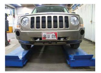
Attachment Tab Height:18"Attachment Tab Width:18"
