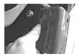
3. Hold the appropriate side bracket to the inside of the frame. Place the bracket butted against the lip of the bumper.
