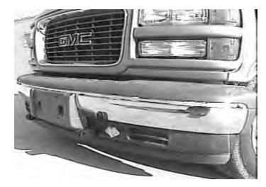
9. Hold the plastic facia piece up to attachment tabs and mark area needed to be trimmed so it can be replaced to its original position.
