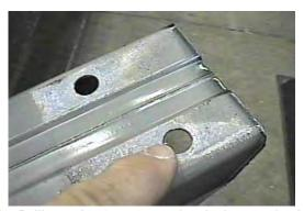
**10.** Drill out the four mounting holes on the back side of metal bumper with a 13/32 drill bit. Install items 6, 7, and 8 with metal bumper and tighten all bolts. **Be sure and use loctite on all bolt before tightening.**
