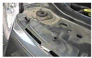
1. Remove the six push pins from the top of grill.
