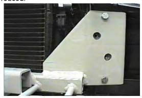
8. Hold baseplate in place so that top edge of end plates are flush with top frame webbing. Use baseplate as a template drill four holes on the front side of baseplate with the 13/32 drill bit. Insert items 3, 4, and 5, do not tighten.
