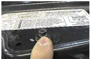
Remove the two metric bolts on the top side grill with 10MM socket. Pull fascia forward and set aside
