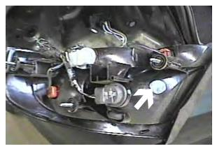
**Note:** If installing the BX8869, Taillight Wiring Kit, Bulb and Socket? This is the recommended location for the hole to be drilled.
