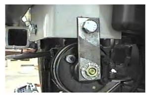
**14.** Reinstall horn use bracket provided, item 9. **Be** sure to use loctite on all bolts before tightening.
