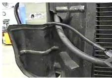
6. Remove two push pins on the air damps both sides and set aside.
