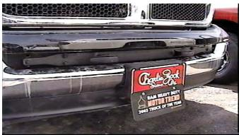
1. For a vehicle with tow hooks, remove the six 15MM bolts to remove the tow hooks. Using existing metric bolts and fasten the baseplate to the truck. Be sure and use loctite on all bolts before tightening. Tighten and torque all bolts according to chart on the General Instruction
