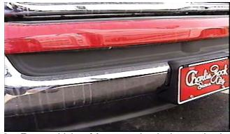
2. For a vehicle without tow hooks has a plastic trim piece that will need to be removed. Once this is removed, bolt the baseplate to existing holes in frame with 1/2-13 x 1 1/2 hex bolts, lockwashers and hex nuts as shown on page 2(items 2, 3 and 4). Be sure and use loctite on all bolts before tightening. Tighten and torque all bolts according to chart on the General Instruction Sheet.
