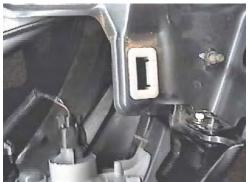
**3.** Just behind headlight assembly is one metric bolts to remove with the 10MM socket, both sides.
