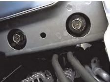
7. Remove two metric bolts from the bottom side of frame rails using the 14MM socket, both sides. Pull metal bumper forward and set aside.
