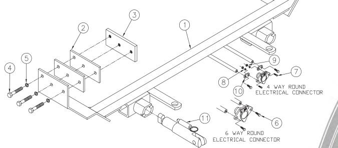
**IMPORTANT:** Use only genuine factory replacement parts on your Base Plate. Do not substitute homemade or nontypical parts. If a bolt is lost or in need of replacement, for your safety and the preservation of your Base Plate, be sure to use a replacement bolt of the same grade (Usually Grade 5, refer to parts list). Repair parts may be ordered through your nearest **Blue Ox** dealer or distributor.
