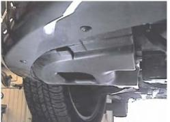
**4.** Forward of front tires remove three push pins on wheel well edge and three on the bottom edge of front fascia, both sides.
