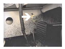
8. Using the 12MM socket, remove one metric bolt from horn bracket on driver's side. Relocate horn bracket straight back on frame rail approximately 1' to existing hole with a nut welded to the inside of the frame.
