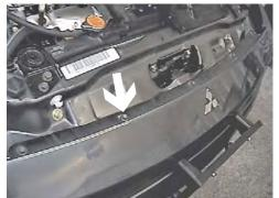
1. Using the 10MM socket, remove the five metric bolts from the top side of front fascia.
