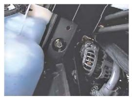
14. Reinstall metal bumper to its original position. Only the back metric bolt will be able to be used on both sides. Be sure and use loctite on all bolts before tightening. Torque all bolts according to torque chart in General Instructions.
