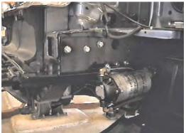
13. Hold baseplate and spacers to align with drilled holes while maintaining a level position with bottom of frame, both sides. Install 3/8" bolts and lock washers on both sides, tighten all bolts. Be sure and use loctite on all bolts before tightening. Tighten all bolts according to torque chart in General Instruction sheet.
