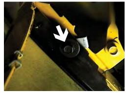
Remove metric bolt from fascia corner, on inside of fender well using the 10MM socket, both sides.
