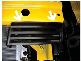
11. Remove two christmas tree clips on lower grill just under metal bumper, set lower grill insert aside. Lower grill insert will NOT be reinstalled.
