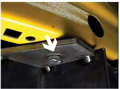
14. On bottom center of metal bumper, align baseplate's (item 1) upper hole, clamp in place with vise grip. Using item 1 as a template, drill upper hole with the 13/32" drill bit, both sides. Insert items 2 into opening on the end of metal bumper to align with drilled hole and tighten items 3 and 4 according to drawing on last page, both sides. Be sure and use loctite on all bolts before tightening. Torque all bolts according to torque chart in General Instructions.
