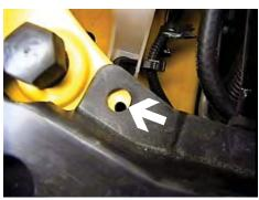
**1.** Remove the seven push pins from the top side of fascia's black plastic cover.
