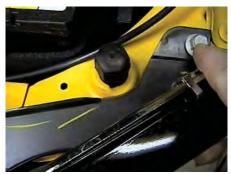
3. Remove two metric bolts from headlight assembly with the 10MM socket, pull forward, unplug electrical and set aside, both sides.
