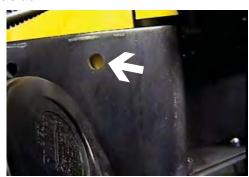
15. Using item 1 as a template, drill all remaining holes on end plates with the 13/32" drill bit, both sides. Insert item 2 into opening on the bottom frame to align with drilled hole. Tighten items 3 and 4 according to drawing on last page, both sides. Be sure and use loctite on all bolts before tightening. Torque all bolts according to torque chart in General Instructions.
