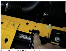
2. Using the 10MM socket, remove the metric bolt on blinker assembly brace, remove one phillips screw, unplug electrical and set aside, both sides.
