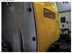
**5.** Just forward of front tire, on wheel well plastic, remove one push pin and two metric bolts with the 7MM socket, both sides.
