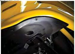
7. Remove the three metric bolts just forward of the front tire, on the bottom side of fascia, both sides.
