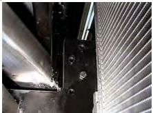
7. Slide baseplate ends to the inside of frame rails. Slide up and forward as far as possible, clamp to frame. Using item 1 as a template, drill the three top holes with the 13/32" drill bit, both sides.
