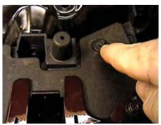
Remove the four metric bolts from the top side of fascia using the 7MM socket. Quad coupe model will not have black cover.
