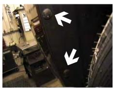
2. Just forward of front tire, inside wheel well, are two push pins to remove and one metric bolt to remove with the 7MM socket, both sides.
