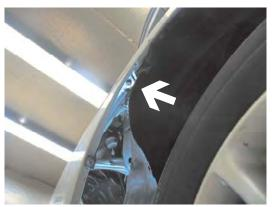
4. Just forward of front tires, on fascia's corner, remove one metric bolt with the 10MM socket, on both sides, pull fascia's corner to the side and forward, set aside.
