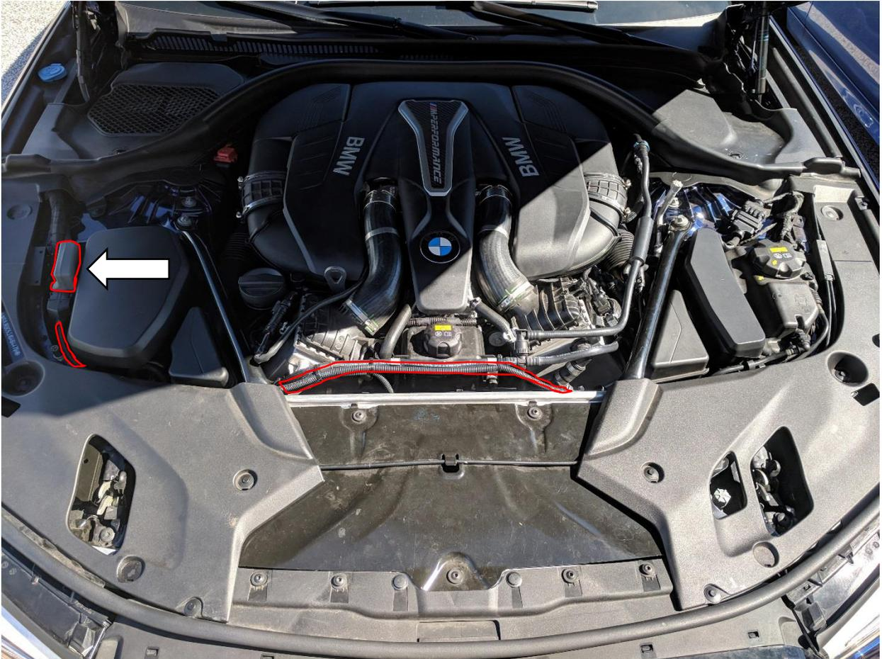
8. If you choose not to mount the DINANTronics Elite ECU in the location shown above, determine a suitable location for the DINANTronics Elite ECU, away from any moving components, water, excessive heat and/or vibration. Route the DINANTronics Elite harness to the desired ECU location, taking care to:
