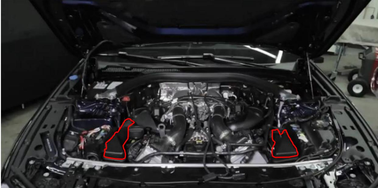
3. Examine the DINANTronics Elite harness supplied with this kit. There are two legs to this harness, which are identical to each other. The DINANTronics Elite attaches to 2 MAP sensors that are located below and in front of the engine (see figures 2-4)
