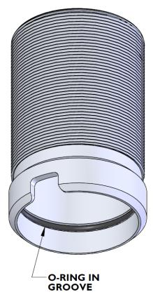
5. See figure below. Slide the threaded sleeves onto the Koni struts as shown. The notch on the sleeve will straddle the swaybar tab.
