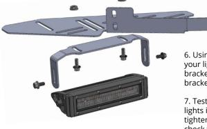
6. Using the included hardware, attach your light bar or pods to the included bracket and then attach it the base bracket.
