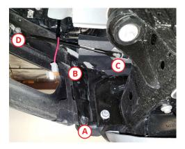
1. Using a 13mm socket, loosen screw (a). Do not fully remove the screw. Next, remove screw (a).
