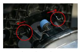
5. Remove the two plastic push rivets shown above that secure the OEM lamp onto the foglight bracket using a trim removal tool (or flat head screw driver).
