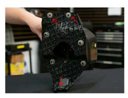
11. Reinstall the entire foglight bracket back onto the vehicle using the three 8mm bolts.
