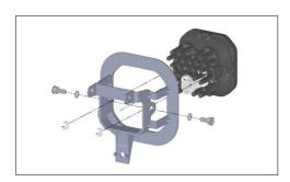
6. Using the included hardware, attach the Type SD bracket to the pod. See the diagram above and make sure the bracket is in the correct orientation. Tighten the bolts down. Do not overtighten or use power tools to torque them down.
