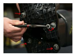
10. Reattach the metal retaining washers.
