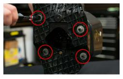
9. Reattach the front bezel using the four 13mm nuts. Do not over tighten.
