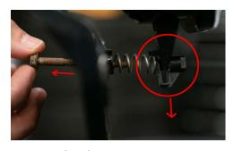
4. Remove the adjustment aiming screw using an 8mm socket.
