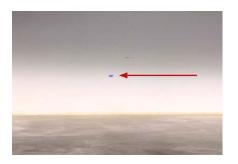
12. Aim your SS3 pods on each side, so that the top of the beam pattern is on the cutoff line mark.
