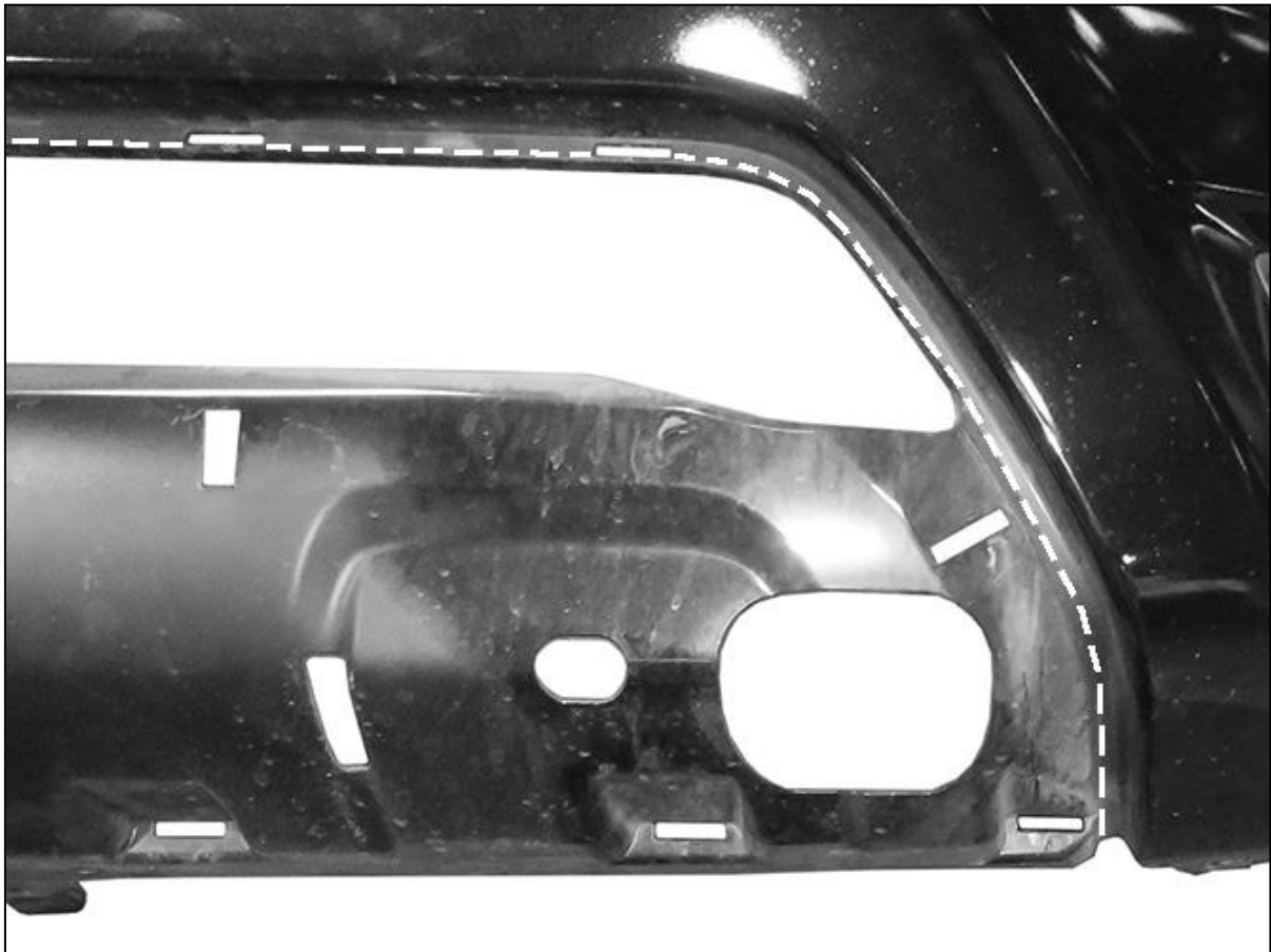
(Fig 12) Use a marker to draw a cut line along the trim line and edge of lip at top. NOTE: Cut edge will be covered with push on Edge Trim. (driver/left side pictured)
