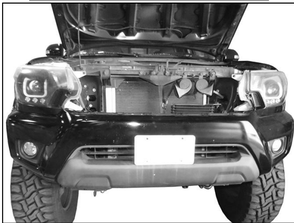
(Fig 3) Remove cover and grille. Remove hardware attaching top of bumper cover to remove cover
