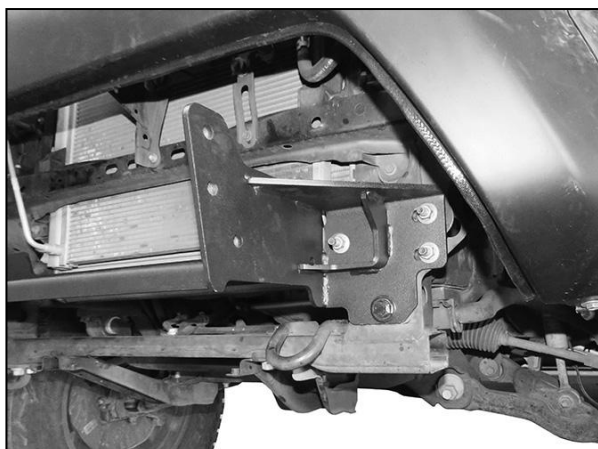
(Fig 14) Reinstall bumper cover. Check fit between bumper cover and Winch Bumper and trim and adjust Bumper as necessary. Clean up rough edges along cut area and push Edge Trim over edge of bumper cover
