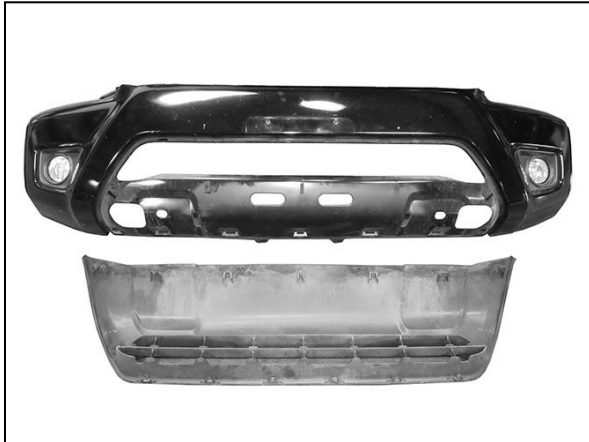
(Fig 10) Lower cover removed
