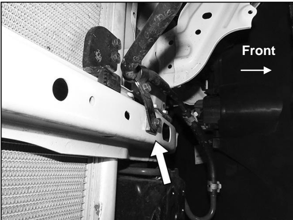
(Fig 7) Reuse hex bolt to attach bracket and Wedge to crossmember
