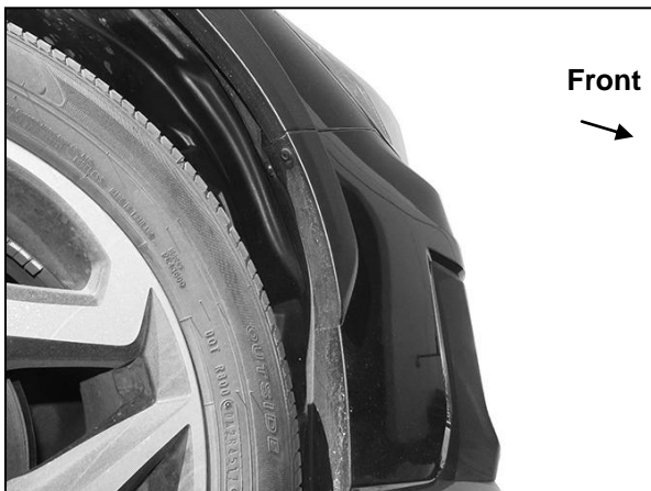
(Fig 1) Remove clips attaching ends and bottom of plastic bumper cover (arrow)
