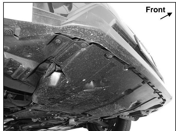
(Fig 2) Remove clips attaching bottom of plastic bumper cover. Remove splash guard from bottom of engine
