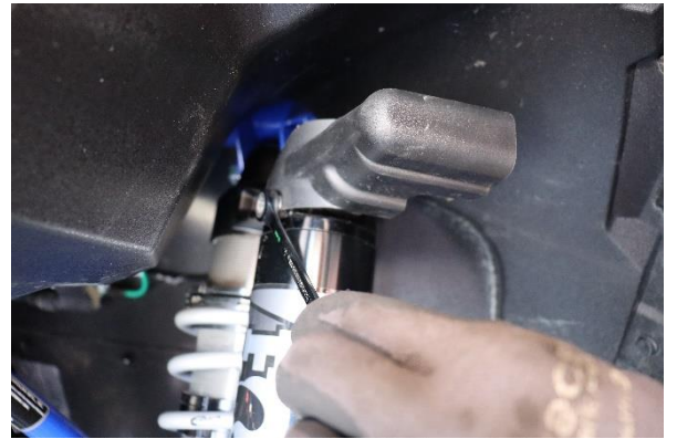
Step 22. Re-install electrical connector cover from the top of the coilover.
