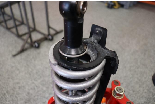
Step 17. Re-install C-clip. When releasing tension off of the spring assembly, make sure spring retainer fully seats on C-clip. Spring retainer locates to the rod end with locating tabs.
