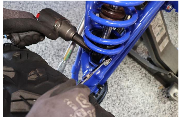
Step 2. Raise the front of the vehicle and support it with the proper safety equipment. Loosen and remove the hardware that secures the coilover to the control arm. Note: Never work on or under a vehicle that is not supported by the proper safety equipment.
