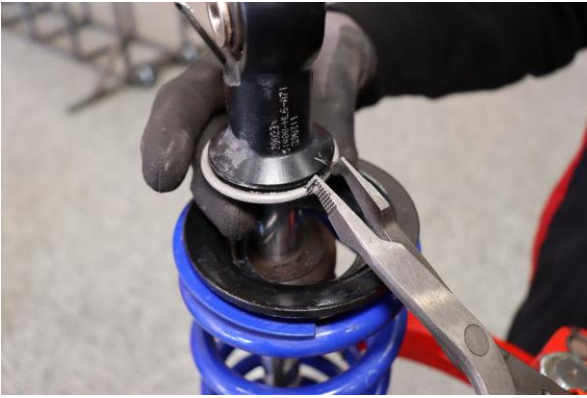
Step 7. Compress the coilover, remove the c-clip . Note: The bump stop will need to be pried down, out of the way of the spring retainer.
