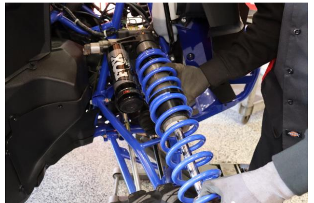
Step 6. Remove the coilover.
