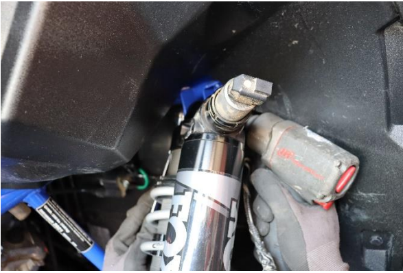
Step 19. Secure the coilover to the upper mount with the OE hardware.
