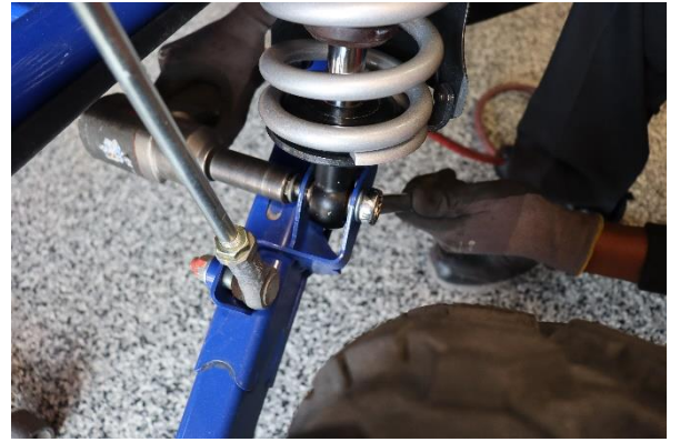
Step 20. Secure the coilover to the control arm with the OE hardware.
