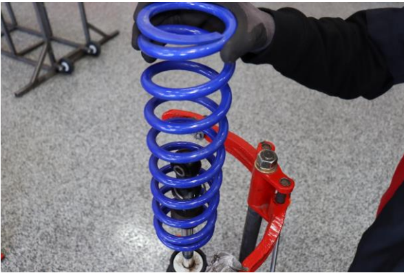
Step 9. Remove OE main spring.
