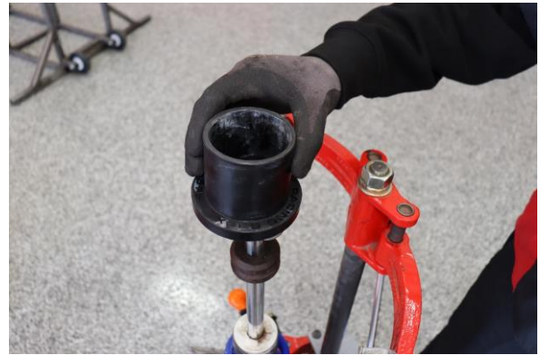
Step 10. Remove OE slider.
