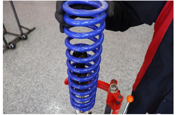
Step 8. Remove OE main spring.
