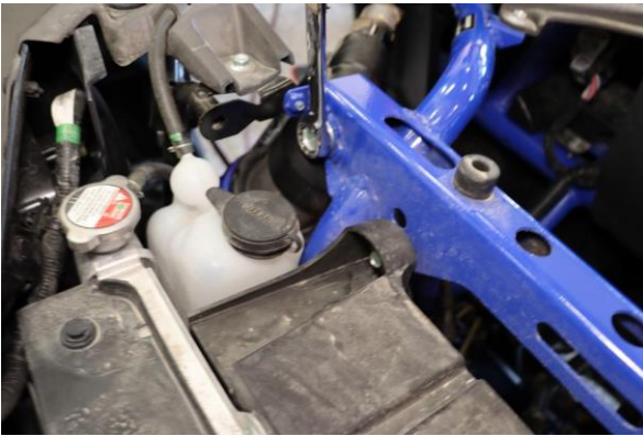
Step 3. Loosen and remove the hardware that secures the coilover to the upper mount.
