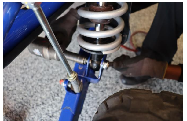
Step 18. Re-install the coilover.
