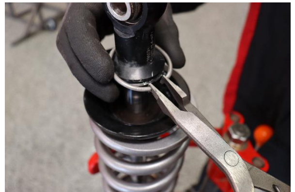
Step 18. Re-install C-clip. When releasing tension off of the spring assembly, make sure spring retainer fully seats on C-clip.
