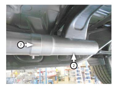
Place clamp (7) onto muffler (3) then connect it to inlet/ extension pipe. Tighten clamp just enough to allow for later adjustment.
