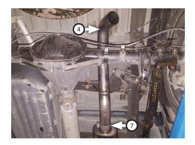
11. Place clamp (7) onto rear tailpipe (5) then connect it to front tailpipe. Insert wire hanger into isolator then tighten clamp just enough to allow for later adjustment.
