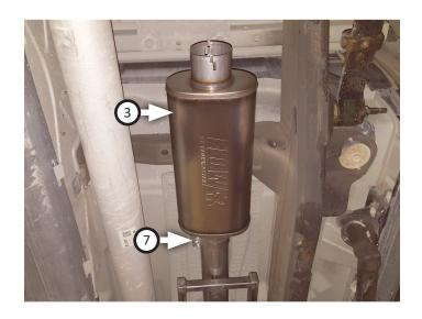
Place clamp (7) onto muffler, route front tailpipe (4)
