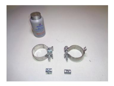
7. Place factory ball clamp (removed step 4) onto **inlet pipe (1)** then connect it to catalytic converter. Insert wire hanger in isolator and tighten clamp enough to allow for adjustment.
