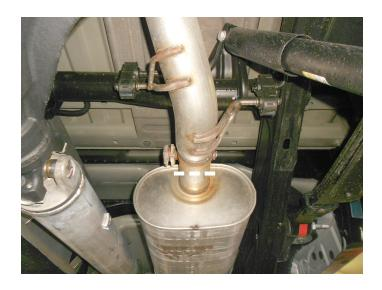
4. Support muffler and disassemble wire hangers from isolators. Loosen ball clamp, disconnect inlet pipe at cat. converter and remove exhaust system. Release tab to remove clamp from pipe and retain it for later use.
