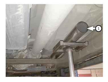
8. If necessary, place clamp (7) onto extension (2) then connect it to inlet pipe. Tighten clamp just enough to allow for adjustment.
