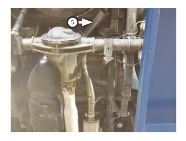
12. Place clamp (8) onto rear tailpipe (6) then connect it to front tailpipe. Insert wire hanger into isolator then tighten clamp just enough to allow for later adjustment.
