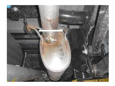
Support muffler and remove all hangers from isolators on muffler assembly; then remove clamp on slip connection just behind catalytic converter. Heat or cut to separate connection and remove muffler assembly.
