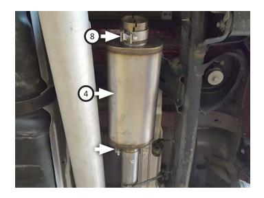
11. Route **front tailpipe (5)** over axle then connect it to muffler. Insert wire hangers into isolators then tighten clamp just enough to allow for adjustment.
