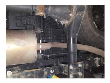
4. Support muffler and disassemble wire hangers from isolators. Remove and retain (x2) bolts from flange then disconnect and remove muffler section from vehicle.
