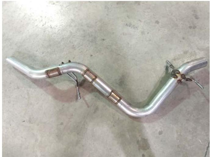
4. Support muffler and disassemble wire hangers from isolators. Measure and cut exhaust pipe 6½" in front of muffler then remove exhaust from vehicle.
