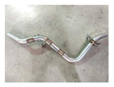
4. Support muffler and disassemble wire hangers from isolators. Measure and cut exhaust pipe 6½" in front of muffler then remove exhaust from vehicle.
