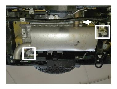
4. Support front pipe then remove flange fasteners. Unbolt isolator mount from frame, separate rear wire hanger from isolator then remove front pipe from vehicle.
