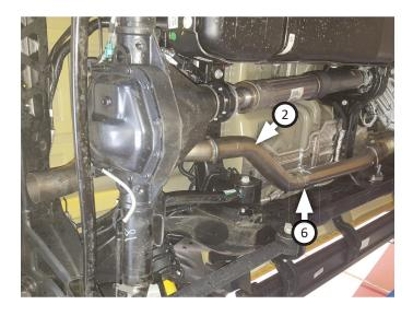
8. Place right rear frame hanger (4) onto passenger isolator over existing factory hanger. Fasten with (x2) lock nuts (14). Place left rear frame hanger (5) onto driver side frame then fasten it with (x2 ea.) bolts (8), lock washers (11), flat washers (10) and nuts (9). Place (x2) rubber hangers (7) onto rear frame hangers.
