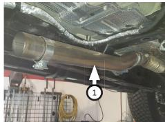
7. Place **clamp (5)** onto **mid pipe (2)** then route it over axle and connect it to inlet pipe. Insert wire hanger into isolater then tighten clamp enough to hold parts.
