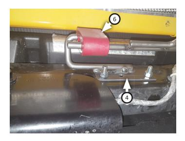
Place clamp (5) onto high exit pipe (3) then connect it to mid pipe. Insert wire hanger into rubber hanger then tighten clamp just enough to allow for later adjustment.
