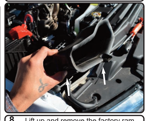
8. Lift up and remove the factory ram from the vehicle.
