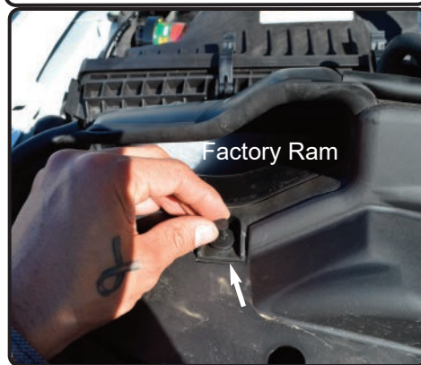
6. Carefully lift up the push clip from OEM factory ram.
