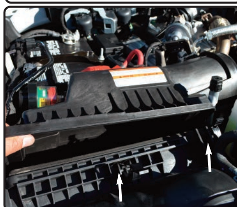
7. Now unclip the upper half of the air box assembly lift up and remove.
