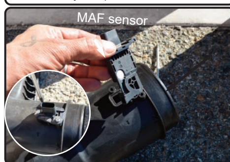
11. Using a T20 torx bit remove the two screws holding in the MAF sensor and remove the MAF sensor.
