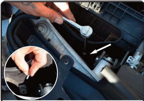
9. Locate the screw holding in the air-box, remove using 8mm socket.
