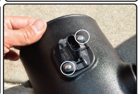
12. Install the MAF sensor into the injen tube and secure using the provided M4 button head screws.
