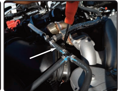
4. Loosen the clamp on the turbo using 7mm nut driver.
