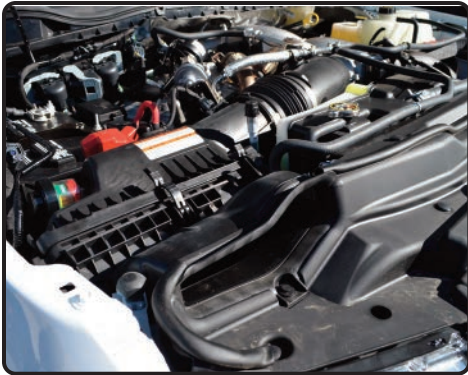
1. Stock intake system shown.
