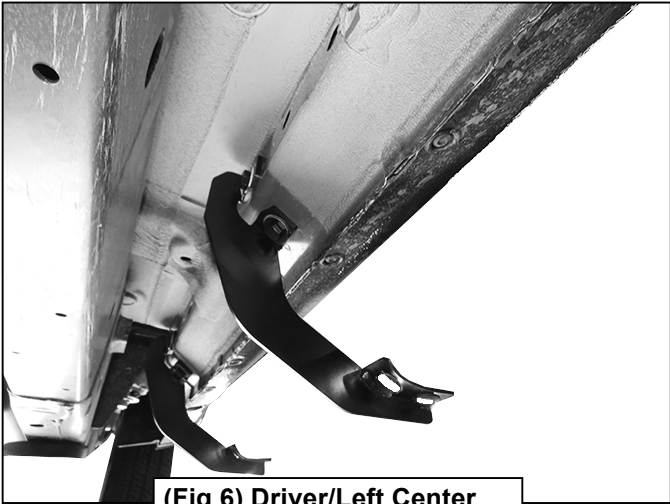
(Fig 6) Driver/Left Center Mounting Bracket installed
