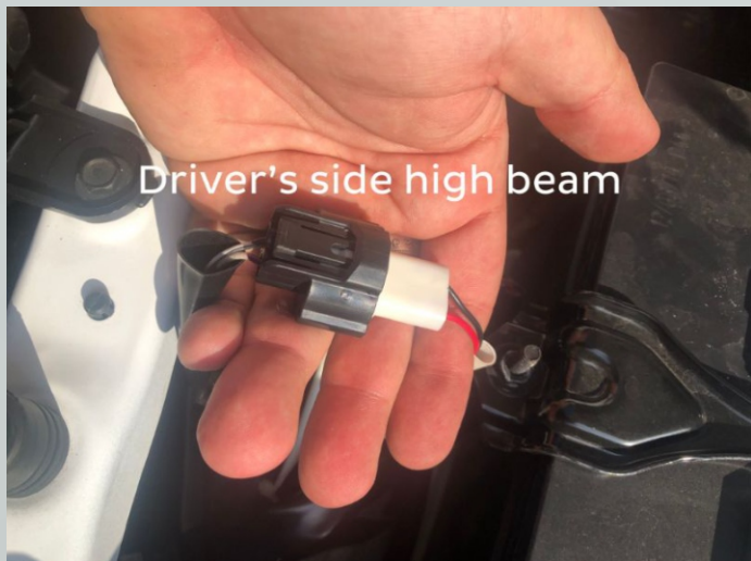
Driver's side (LH) high beam - Black to white w/ black stripe
