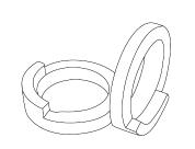
**2x OPTIONAL Large protective sleeves** - these fit around the large adjusters
