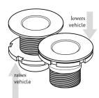
2x Combined adjusters to couple the black and orange springs together and adjust height
