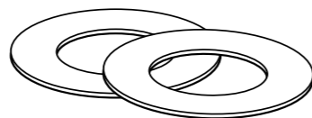
2 MSS supplied rubber centralising ring to eliminate side ways movemnt through the system x
