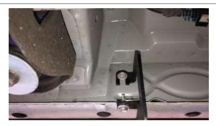
**<u>Step 8</u>**: There will be  $\frac{1}{2}$ " of adjustment in the (x3) mounting bracket. Adjust to desired position and tighten to (20 ft,/lbs).
