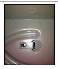
Step 6: Align the Nerf Board with the mounting holes. Beginning with the middle bracket, use one M8-1.25 bolt and one fender washer for each mounting location and thread the bolts into the mounting holes and leave loose. Continue with the front and rear bracket. NOTE: Some vehicles require the use of an additional nut and washer for the lower portion of the mounting bracket.
