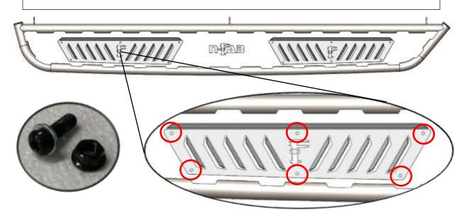
**Step 3:** Install the supplied rocker panel brackets (x6) to the attachments points located on the backside of the main tube (Driver/Passg) using the supplied 3/8" x 1" carriage bolts and 3/8" flanged nuts. Leave finger tight for now.
