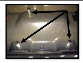
**Step 5:** Install Nerf Board assembly to the factory mounting location using the supplied M8 flanged hex nut and flat washer (x9). Leave loose for now.
