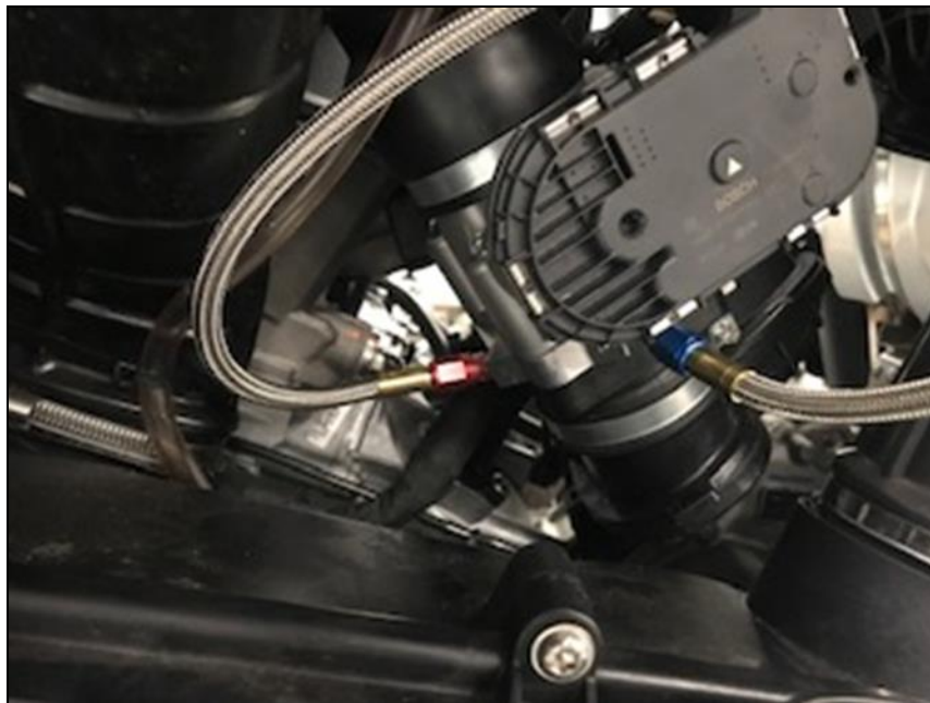
Figure 10 – Nitrous Plate Installation
