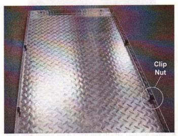
Snap clip nuts into the square holes located in the sides of floor pan. Note the clip nuts should be located on the inside of the floor pan as shown above. (Important: Do only the four side holes at this time.)
