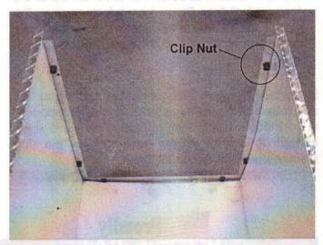
4. Place interior liner in floor and side panels as shown above. Push liner firmly in place and snap clip nuts into square holes located in both ends of side panels. Note: Liner should be behind clip nuts as shown.
