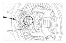
**24.** Verify spacer paddle is aligned with the paddle opening in synchro ring and press down on driver/spacer to seat on coupler; driver teeth should be fully engaged all the way around.
