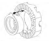
**21.** Insert the other active spacer into the other driver. Seat the spacer paddle at the paddle opening (missing extended tooth).
