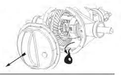
7. Remove the axle retaining bolts located on the inside of the brake backing plates. Pull out both axle shafts approximately 8".
