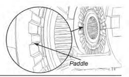
**18.** Insert an active spacer into a driver. Seat the spacer paddle at the paddle opening (missing extended tooth).
