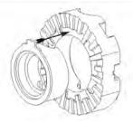
**19.** Insert driver/spacer as shown, making sure spacer paddle is facing out towards you.
