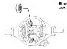
**15.** Install coupler inside differential case, ring gear side first.
