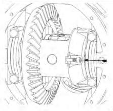
**38.** Insert retaining bolt/roll-pin into case/shaft. Tighten retaining bolt firmly.
