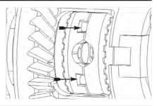
**25.** Wedge both drivers in engagement with couplers. Rotate driver's side wheel forward 1/4 turn to reveal spring slot.
