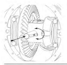
**37.** Using the retaining bolt/roll-pin as a handle, insert the shaft into the differential. Press hard while twisting to pass shaft by springs.
