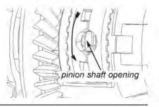
**35.** Feel through pinion shaft opening and verify both spacers and drivers are fully seated onto couplers. Verify all 8 saddle springs are fully seated in holes.
