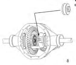
**17.** Make sure paddle opening (widest gap) in ring gear side synchro ring is facing out towards you.
