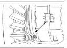
31. Visually inspect notches in spring slot to make sure inner spring is fully seated.
