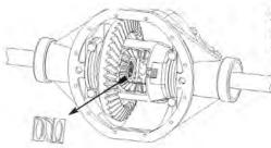
**9.** Remove clutch spring (some may have multiple coil springs) if present.
