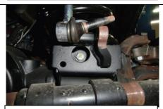
Remove lower shock mounting bolt located below spring
