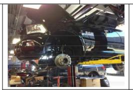
Lift the vehicle by the frame. Support the axles and remove the tires.
