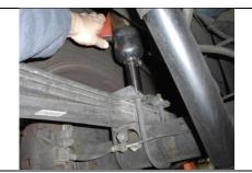
Work on one side of vehicle at a time, remove rear u-bolts.
