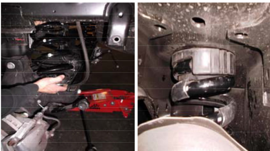
Reinstall the coil spring with the spacer.
