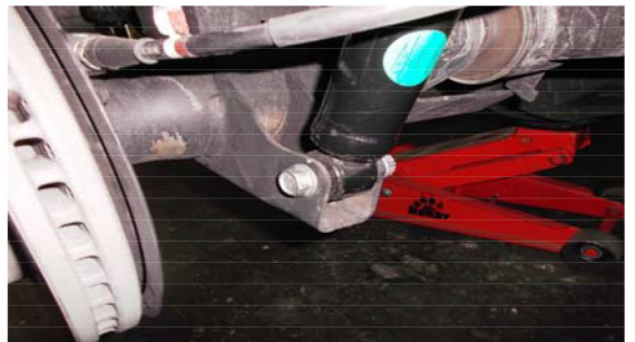
Jack the axle back up to weight the springs then install the shocks.
