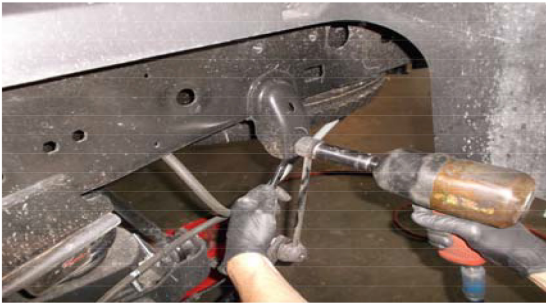
Unbolt the sway bar end links.
