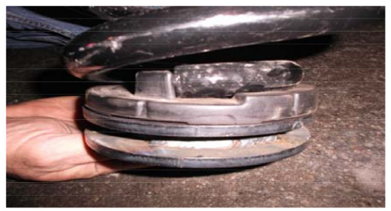
Place the coil spacer under the lower spring isolator.
