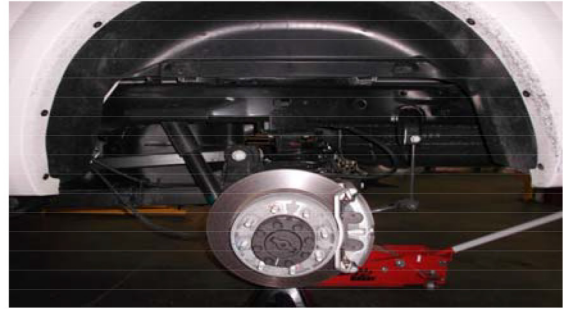
Lift the vehicle by the frame, support the axle, and remove the wheels.
