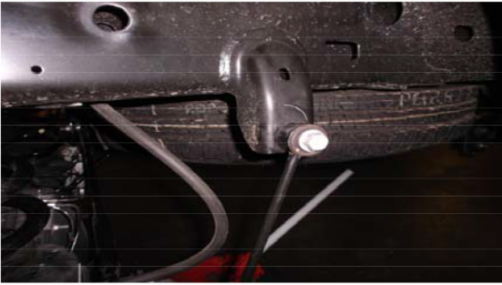
Reinstall the sway bar end links.
