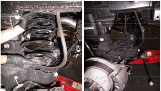
Lower the axle until the springs are loose enough to remove.
