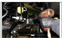
Support rear suspension and remove rear trac bar bolt
