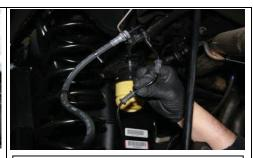
Disconnect ABS lines to avoid damage during installation.
