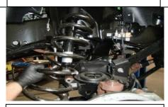
Reattach shocks, trac bar, sway bar end links, and ABS lines
