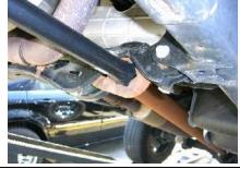
Remove the torsion key adjusting bolt. Using a Torsion Bar Unloading Tool relieve the pressure on the key way. Remove the threaded part of the torsion adjuster. Release the tension on the unloading tool
