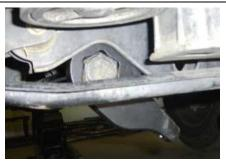
Install the new torsion key and slide torsion bar back into position. Using Torsion Bar Unloading Tool, create enough space to reinsert the torsion key adjuster.
