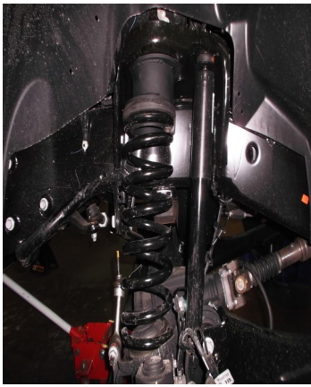
Install the assembly in to the vehicle. Note: Coil Spacer position. Coil Spacer Should be orientated so the spring is offset to the front of the coil pocket and to the inside of the frame to correct "Spring Bowing"
