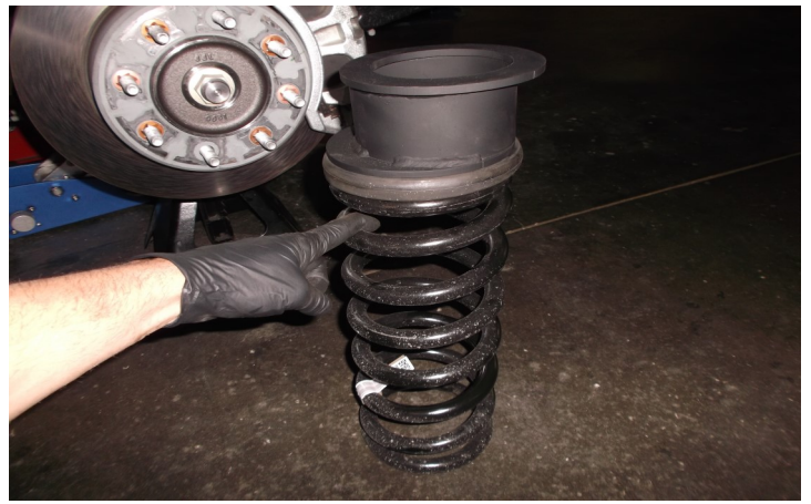
Install the OE spring isolator and the strut spacer onto the coil spring. Lower the axle further to allow spring installation.
