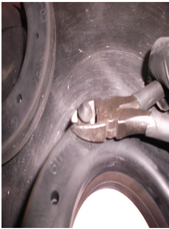
On OE spring isolator, cut off the rubber locating tab
