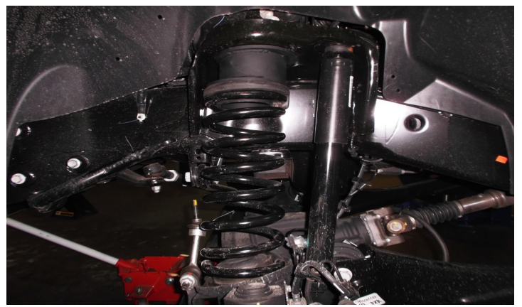
Raise the axle to weight the springs.
