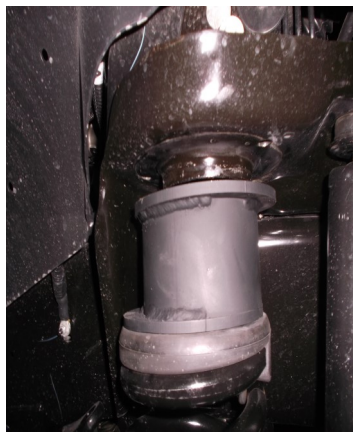
Install the assembly in to the vehicle. Note: Coil Spacer position. Coil Spacer Should be orientated so the spring is offset to the front of the coil pocket and to the inside of the frame to correct "Spring Bowing"
