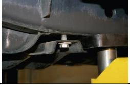
Loosen (2) front transfer case skid plate bolts.
