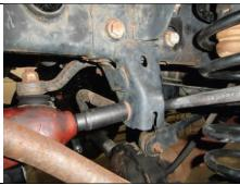
Support front axle and remove upper trac bar bolt.
