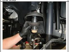
Remove the upper spring isolator to expose mounting hole
