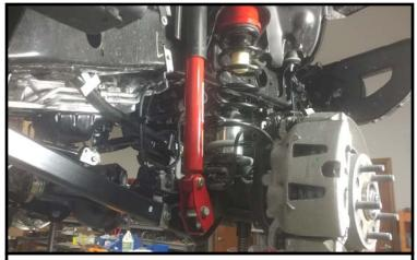
Install the brake line brackets to the frame and control arm using the factory hardware.
