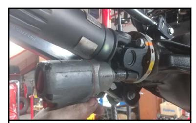
Install the front drive shaft to the pinion using the previously made marks and factory hardware. Use thread locker and tighten.
