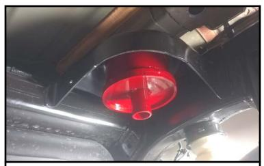
Install the spring spacer using the provided hardware to the nut plate.
