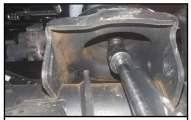
Install the bump stop hardware and tighten.
