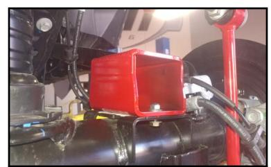
Install the rear bump stop extensions using the provided hardware. Install the wheels and lower the vehicle to the ground. Have the align set.
