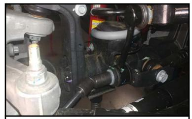
Remove the lower sway bar end links from the axle.
