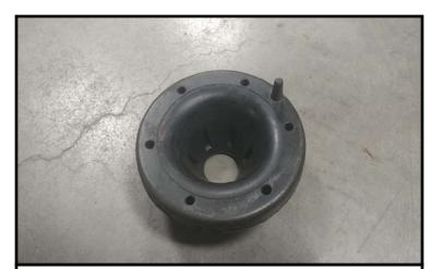
Cut the nipple off the rubber isolator.
