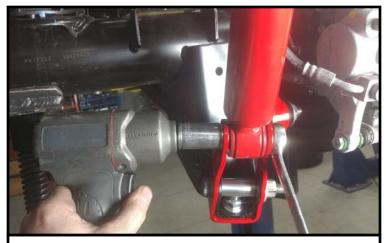
Install the shock to the shock extension using the provided 1/2" hardware. Install the provided crush sleeve and factory hardware.
