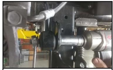
Install the lower sway bar end link to the axle using the factory hardware.
