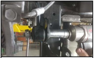
Remove the lower sway bar end link from the axle. Lower the axle enough to remove the springs and isolators.
