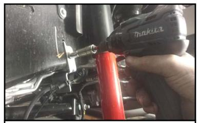
Jack the vehicle up from the front axle. Support the vehicle with jack stands under the frame. Remove the brake line bracket at the frame.
