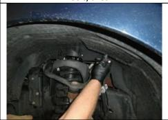
Loosen upper strut mount nuts.
