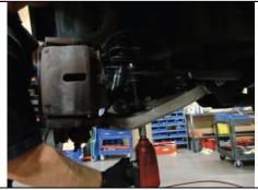
Remove lower sway bar end link hardware.
