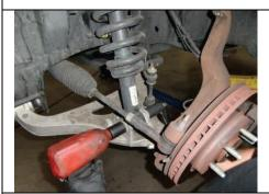
Loosen lower strut bolt/nut and remove.
