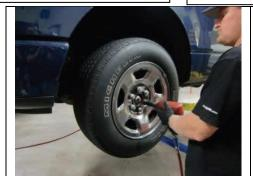
Lift vehicle securely and remove wheels/tires.
