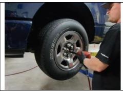
Lift vehicle securely and remove wheels/tires.
