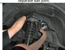
Remove top strut mount nuts and remove assembly.
