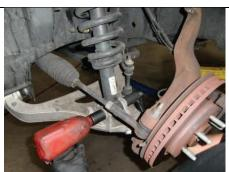
Loosen lower strut bolt/nut and remove.
