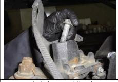
Remove bolt from middle of spring perch
