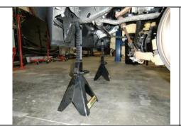
Lift front of vehicle and support with min. 3 ton jack stands.
