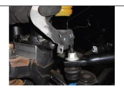
Bend tab 180 degrees so line will relocate behind bracket
