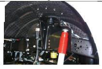
Carefully lower axle and remove coil spring
