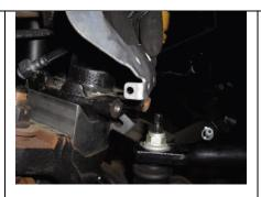
Then reconnect vacuum line and clip and reattach bracket
