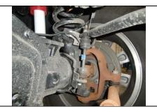
2011-UP Disconnect lower sway bar mounting hardware
