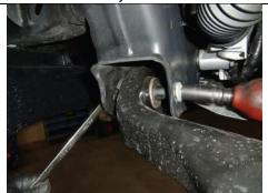
Loosen and remove front lower control arm bolt and nut
