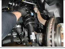
Remove strut assembly from vehicle
