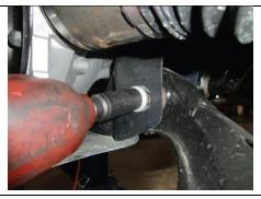
Loosen and remove rear lower control arm bolt and nut.
