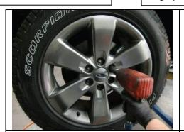
Raise and support front of vehicle off the ground. Remove front wheels/tires, support suspension with jack.
