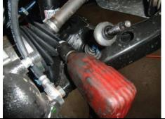
. Disconnect and remove lower shock bolt and nut.
