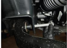
Torque lower control arm hardware at ride height. Lift lower control arm into position and reinstall bolts.
